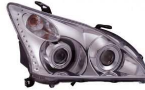
LE057-A11011MN CHROME HOUSING & PROJECTOR W/REFLECTOR & CCFL
